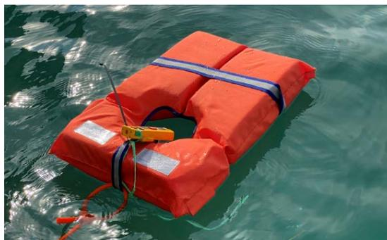
Figure 1. PLB M100 transmitter attached to the life jacket
