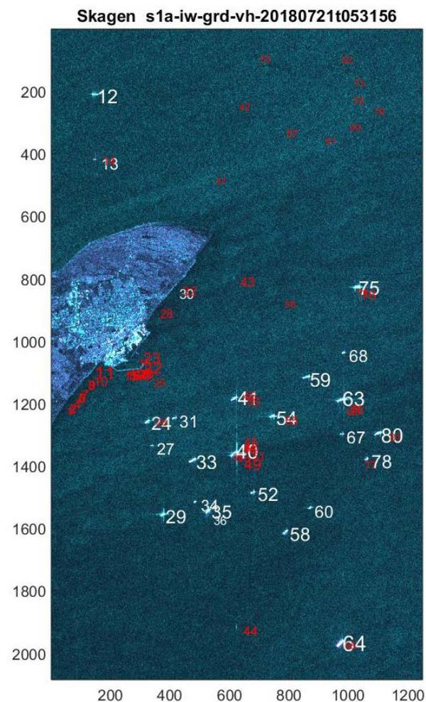
Figure 2. Copernicus Sentinel-1A image [August 21<sup>st</sup>, 2018 at 05:32 a.m. UTC] covering Skagen, the northern tip of Denmark. The added numbers refer to the list of objects found by the classification algorithm, where white numbers are ships and red numbers are mostly wakes, sidelobes, and harbor piers.
