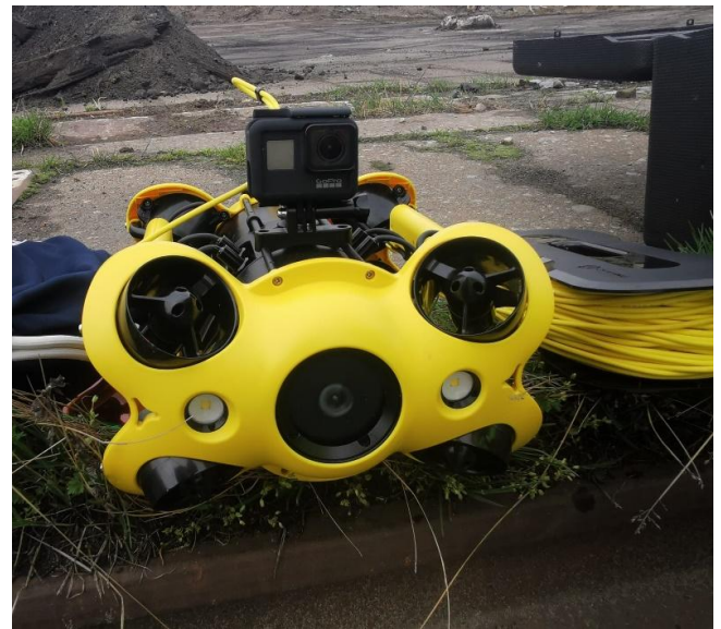
Figure 1. Chasing M2 - ROV with GoPro camera used in experiment
