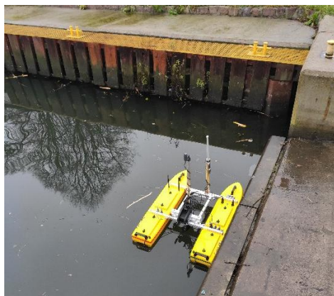
Figure 1. Autonomous surface vehicles (USV) prepared for bathymetric survey on the Odra River, Szczecin.
