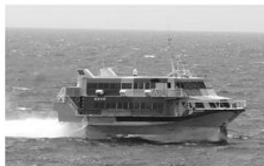
Figure 1. Hydrofoil type of high-speed vessel, which are used for important high-speed sea routes linking remote islands with the Japanese mainland. (Photograph by H. Kato)
