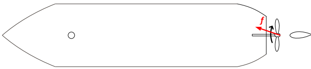
Figure 3b. Resultant force for the vessel moving ahead
