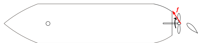
Figure 2b. Resultant force for the vessel altering its course to port
