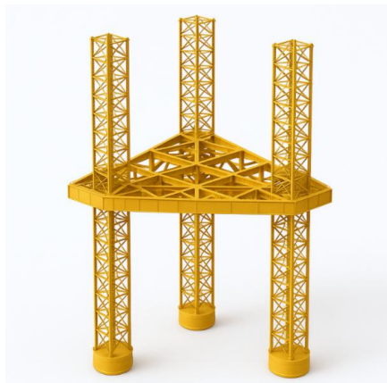
Figure 1. Simplified 3-D model of typical three-legged jack-up hull-leg assembly (based on [28] AI generated).
