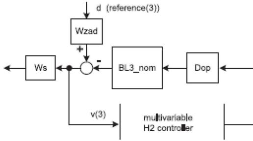
Figure 10: The block diagram of the augmented open-loop process for H<sub>2</sub> controller synthesis. Symbols denote: BL3 nom - state model of the control object; Dop - adaptation matrix; Wzad - filters for reference signals; Ws - weighting functions for control performance. Numbers in parentheses denote sizes of the signal vectors.
