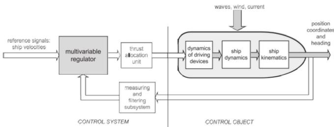
Figure 2: The block diagram of the multivariable ship control system.
