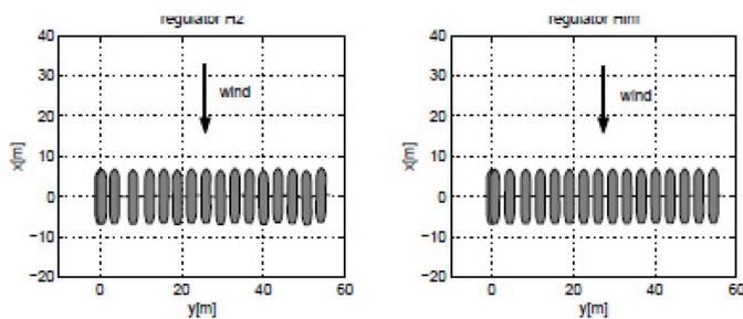
Figure 12: The trajectory of the ship in the first example drawn by silhouettes every 60[s]. Initial heading  $\psi_0 = 0[\text{deg}]$ , the trial period  $t = 1000[\text{s}]$ . An arrow indicate the average wind direction.
