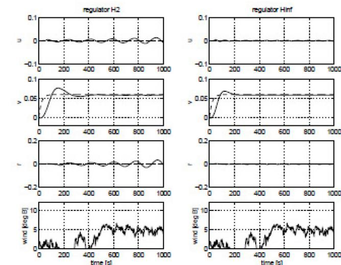
Figure 13: The velocities of the ship in the first example - from the top: surge, sway and yaw. The bottom figures present the wind speed in Beaufort scale (recalculated in the ship model scale 1:24). Solid lines denote real values, dashed lines - commands.
