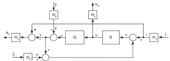
Figure 3: The block diagram of the closed-loop system with weighting functions for selected signals. The meaning of the particular signals is as follows:  $\tilde{r}$  - references vector,  $\tilde{p}$  - vector of disturbances,  $\tilde{n}$  - noises vector,  $\tilde{e}_y$  - weighted control errors,  $\tilde{e}_u$  - weighted control signals.
