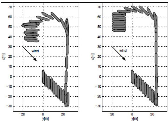
Figure 18: The trajectory of the ship in the third example drawn by silhouettes every 60[s]. Initial heading  $\psi_0 = 0[\text{deg}]$ , the trial period  $t = 2800[\text{s}]$ . An arrow indicate the average wind direction.
