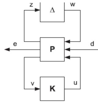
Figure 5: The generalized closed-loop system configuration with uncertainties.
