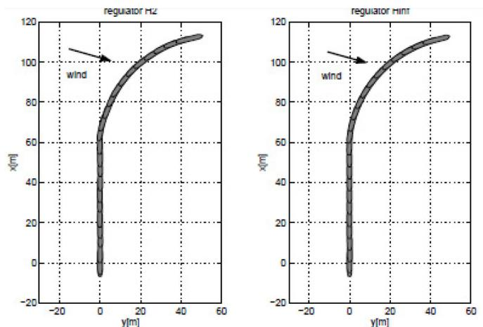
Figure 15: The trajectory of the ship in the second example drawn by silhouettes every 60[s]. Initial heading  $\psi_0 = 0[\text{deg}]$ , the trial period  $t = 1400[\text{s}]$ . An arrow indicate the average wind direction.
