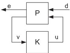
Figure 4: The generalized closed-loop system configuration.
