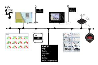
Figure 1. CAN bus interconnection of (clockwise, from upper left) the weather station, AIS and GNSS receivers, gyroscope, compass, navigation display, myriad sensors, VDR, and ship state dashboard display.
