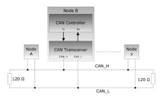
Figure 2. CAN bus nodes connected to the two-wire bus. Note that the bus is terminated with a resister. (Source: https://cdn10.bigcommerce.com/s-7f2gq5h/product\_images/uploaded\_images/can-bus-network-with-transceiver.jpg)
