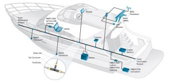
Figure 6. Maritime instrumentation and the NMEA 2000 bus on a boat. (Source: https://upload.wikimedia.org/wikipedia /commons/b/bf/NMEA2000\_Modified\_motor\_yacht.jpg)
