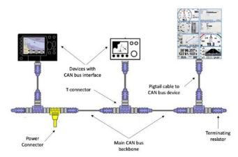
Figure 3. CAN bus architecture.
