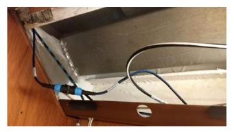
Figure 10. Easy physical access to the CAN Bus on a vessel can make it simple to add a rogue device.
