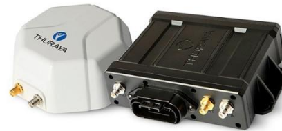
Figure 6. Thuraya T2M-DUAL. Source: User & Installation Manual Thuraya Satellite Communications System
