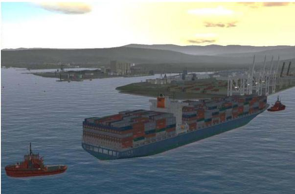
Figure 8. Fully loaded container vessel (111626 DWT) approaching terminal with assistance provided by pilot and two tugs – wind 5 knots from 060°
