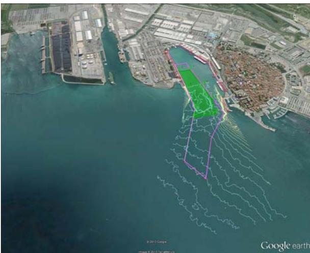
Figure 9. Final layout – the green sector shows the minimum required width based on statistical analyses and a 95% confidence level at various metocean conditions.
