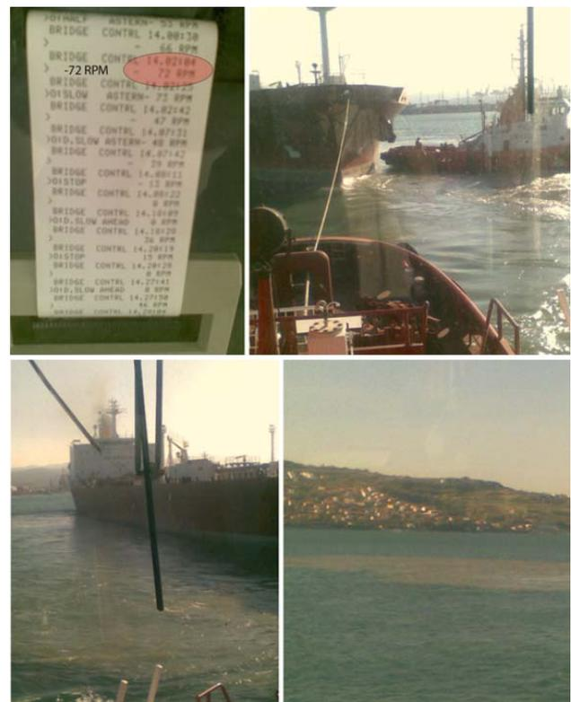
Figure 10. Intrusive manoeuvre "full astern" resulting in extensive propeller wash
