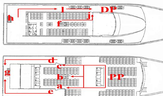
Figure 2. Escape routes arrangement together with the direction of the evacuation
