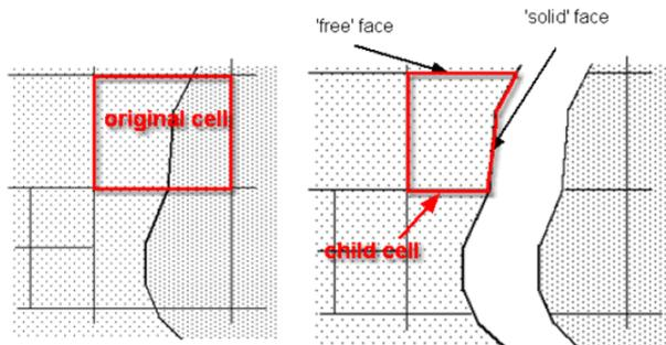
Figure 10. Sub-grid resolution of curvilinear wall (FlowVision 2010)
