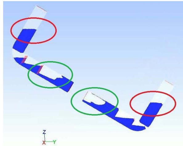
Figure 6. The surface of liquid sloshing in partly filled high side tanks (Krata, Wawrzyński, Więckiewicz, Jachowski 2012)
