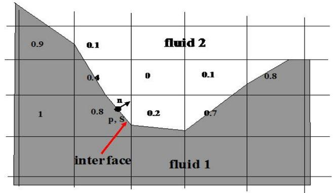
Figure 11. VOF (Volume Of Fluid) variable is the volume fraction of fluid 1 in a cell; VOF=1 - the cell contains only fluid 1; VOF=0 - the cell contains only fluid 2;  $0 < \text{VOF} < 1$  the cell contains fluid 1 and fluid 2 (FlowVision 2010)
