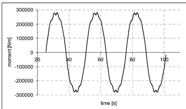
Figure 15. History of heeling moment  $M_{Total\_dyn}$  due to liquid sloshing in the considered tank –sample case
