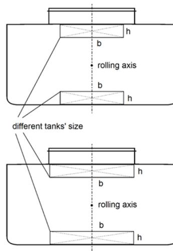
Figure 8. Arrangement of considered tanks in ship's hull
