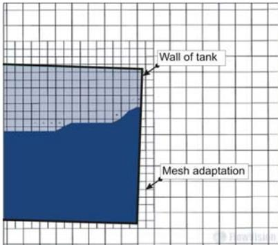
Figure 9. Computational mesh and two coupled reference frames systems
