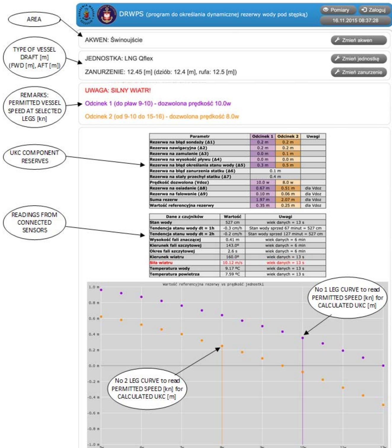
Figure 6. Graphical user interface for dynamic UKC
