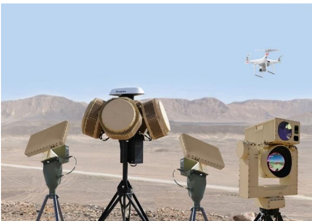
Figure 10. DRONE DOME system [52].
