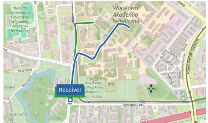
Figure 7. Spoofing UAV position using dynamic attack.
