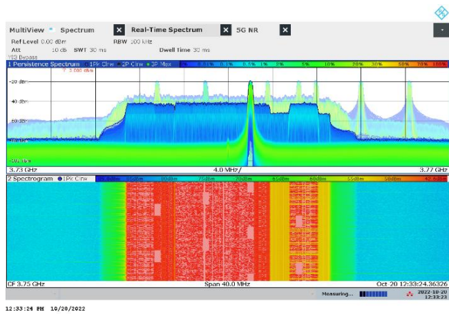
Figure 5. Example of 5G channel jamming using sweep noise technique with sweep rate of 10 changes per second [27].
