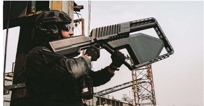
Figure 8. Handheld DRONESHIELD DroneGun Tactical system [50].
