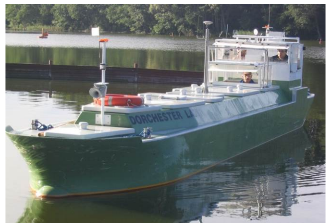
Figure 1 The manned model representing a large LNG carrier used for training and research purposes
