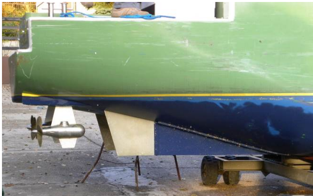
Figure 4. The LNG carrier model equipped with two pulling azipods used for stopping tests (in this photo the pulling azipods are turned around by 180 degrees)
