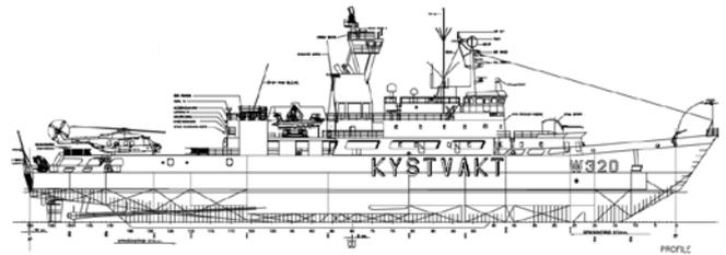
Figure 6. KV Nordkapp's profile from the GA plan.
