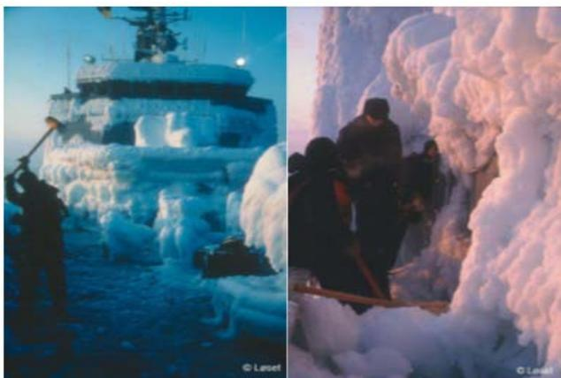
Figure 1. Icing on Coast Guard vessel KV Nordkapp on 27 February 1987, Barents Sea (Photo by Prof. S. Løset).
