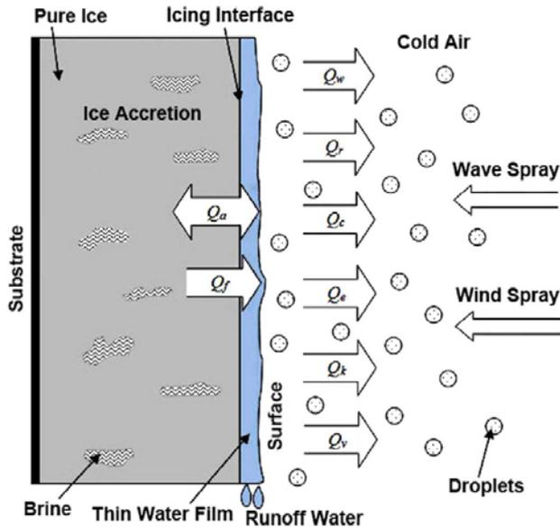
Figure 3. Schematic illustration of the relationship between sea spray icing and heat flux balance (Dehghani-Sani et al., 2017)
