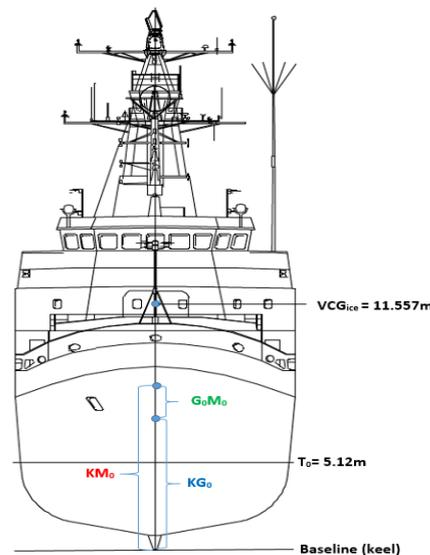
Figure 7. KV Nordkapp from the GA plan of the ship, showing the center of gravity of accumulated ice ( $VCG_{ice}$ ), initial vertical center of gravity ( $KG_0$ ), initial depth ( $T_0$ ),
