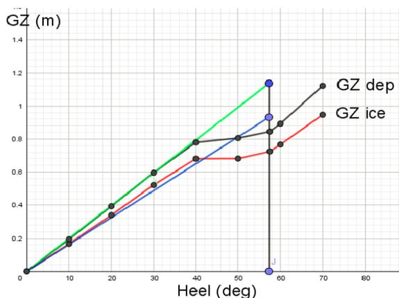
Figure 8. KV Nordkapp's GZ curve based on departure and ice accreted conditions, February 26 and 27 1986.
