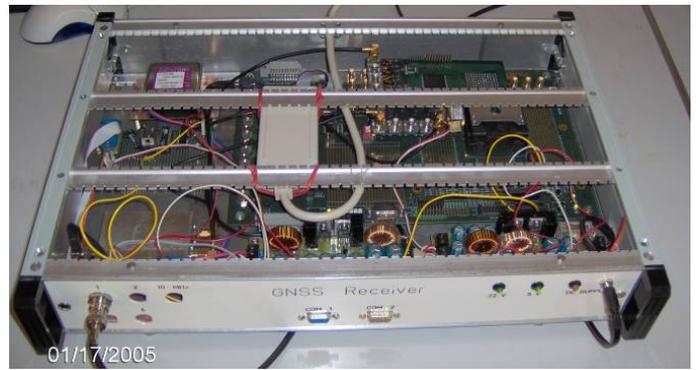
Fig. 3. Experimental GNSS Receiver in 19-inch rack
