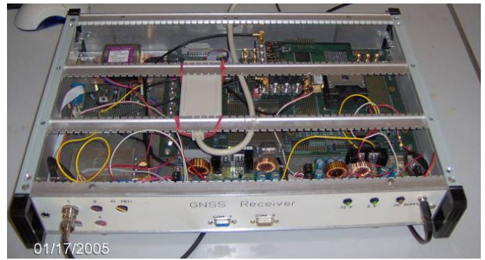
Fig. 3. Experimental GNSS Receiver in 19-inch rack
