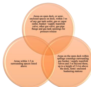
Figure 8. Determination of Hazardous areas on board
