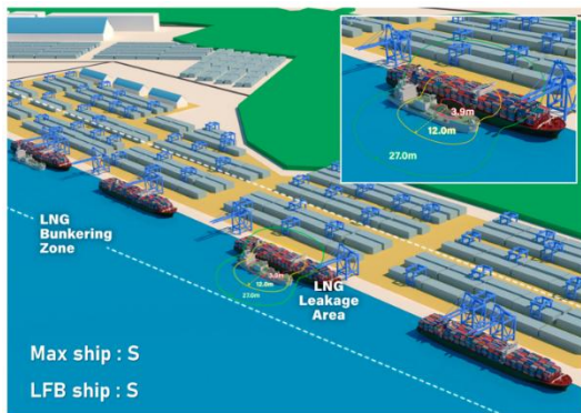
Figure 7. Restricted areas during LNG bunkering
