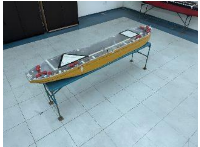
Figure 4. Mechanisms (mooring elements in red) and markers (triangle and rectangle in white) installed on the ship's deck for unintentional unberthing simulation.
