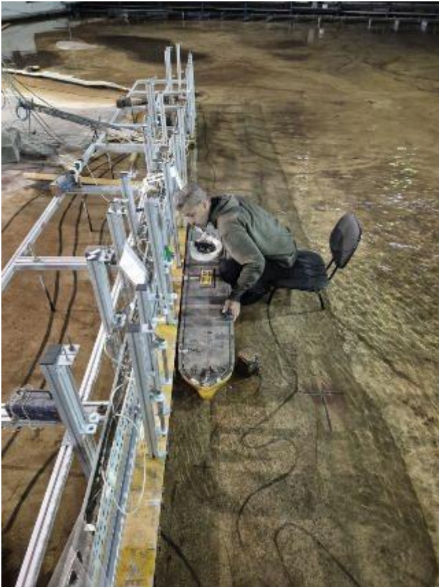
Figure 3. Ship positioning process at the center of the berth.
