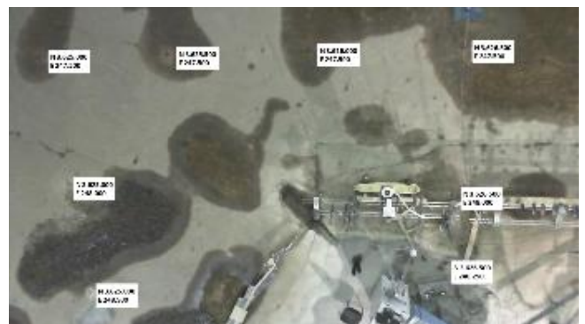
Figure 6. Image of the vessel's position monitoring system, highlighting reference points with known coordinates (in meters).
