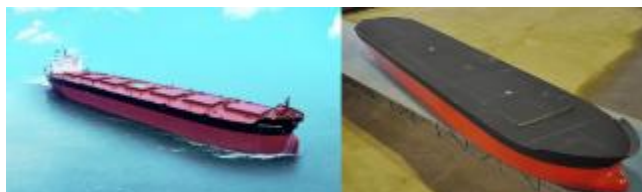
Figure 1. View of the real 400,000 DWT VLOC (left) and its 1:170 scale model (right).
