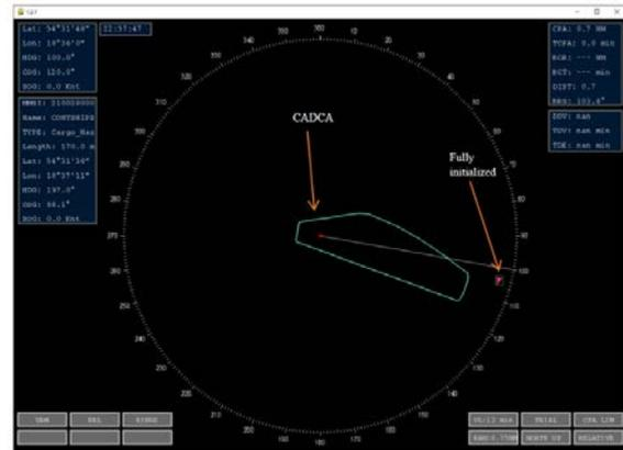
Figure 7. Collision Avoidance Dynamic Critical Area (CADCA)
