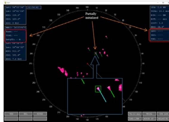
Figure 8. Acquisition of partially initialized target ship
