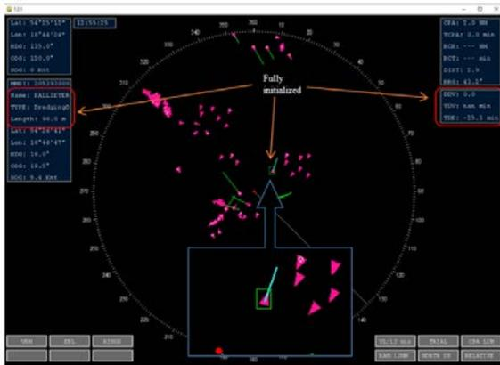
Figure 6. Acquisition of fully initialized target vessel
