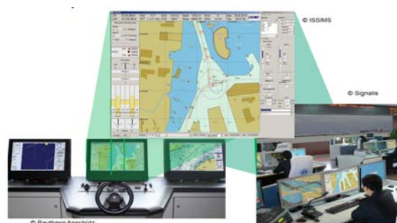
Figure 7. Project COSINUS – shared information on manoeuvring plans and multiple prediction in ECDIS between bridge and VTS
