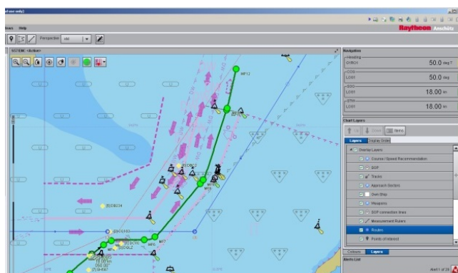
Figure 8. Project COSINUS results: Display of manoeuvring plan (green) of own ship together with route plan of another vessel (blue) presented in Integrated Navigation System of project partner Raytheon-Anschütz transmitted from VTS station of partner SIGNALIS
