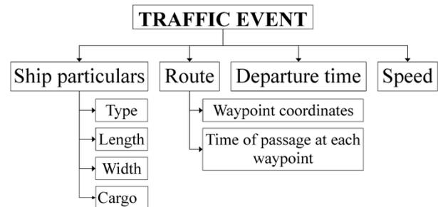
Fig. 3. Generated data for each simulated vessel (traffic event)
