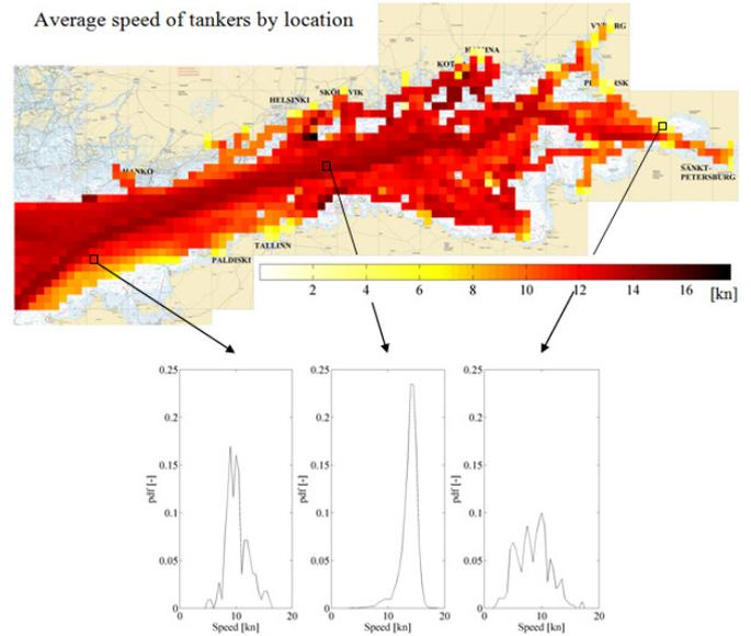
Fig. 8. Average speed of tankers in the Gulf of Finland and local speed distributions, based on AIS data of 2006-2009
