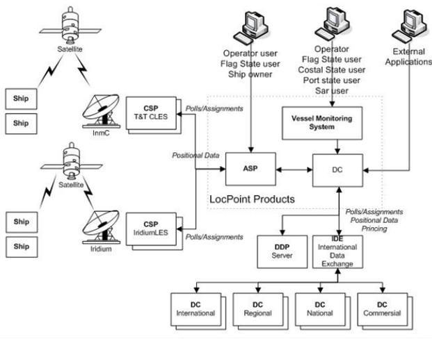
Fig.3. Global Ships Monitoring System
