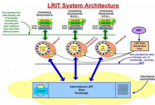
Fig.1. LRIT System Architecture
