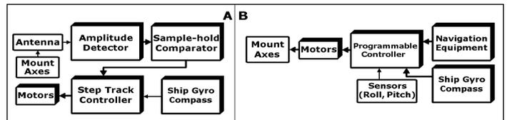
Figure 5. Functional Block Diagrams of Step and Program Tracking
