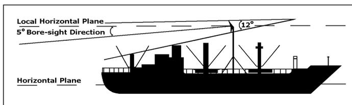
Figure 7. Theoretical Antenna Installation
