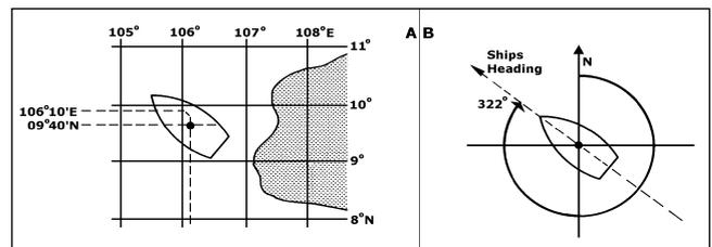
Figure 10. Antenna Pointing Courtesy of Manual: "Saturn 3" by EB Communications [04]
