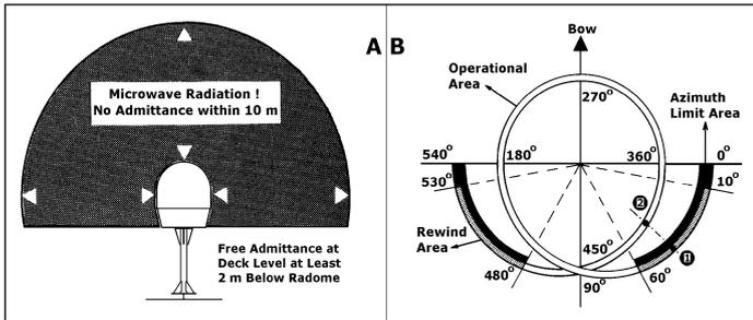
Figure 9. Antenna Radiation Precautions and Azimuth Limit Courtesy of Manual: "Saturn 3" by EB Communications [04]
