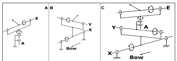
Figure 3. Two and Four-axis Mount Systems
