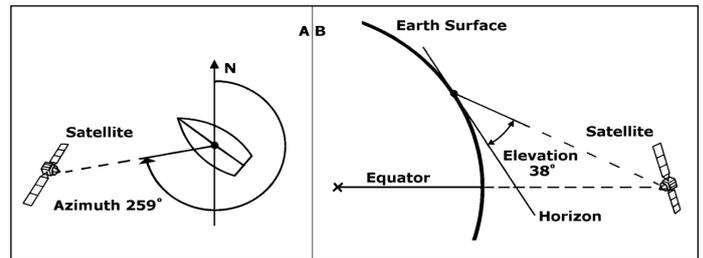
Figure 11. Azimuth and Elevation Angle
