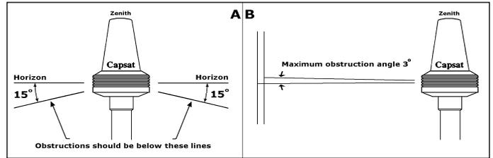
Figure 6. Safe Distance of Inmarsat-C Antenna from Obstructions
