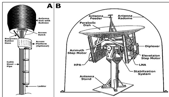
Figure 8. ADE Mast and Stabilized Platform
