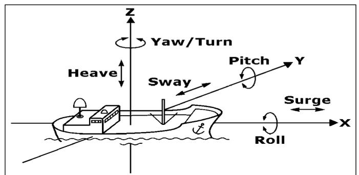
Figure 2. Components of Ship Motion
