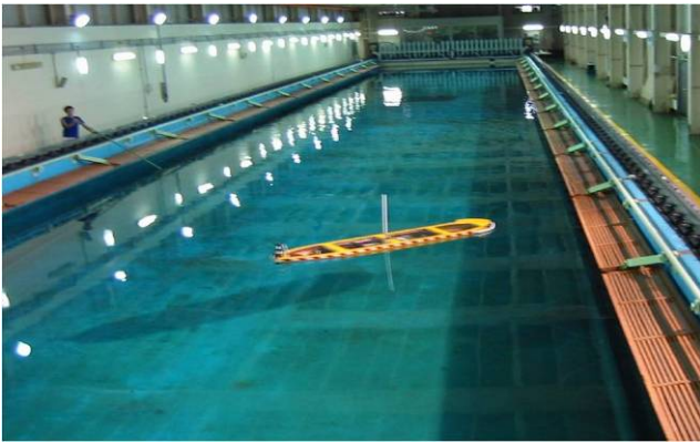
Figure 10. Zig-zag test in towing tank
