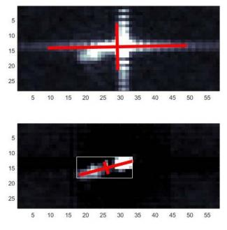
Figure 3. Top: S1 SAR image of the container ship Ivar Reefer in Fig.2. Ship dimensions are 164x26m but show strong sidelobes. Bottom: sidelobes have been removed. Red bars show the resulting and improved ship length, breadth and direction.
