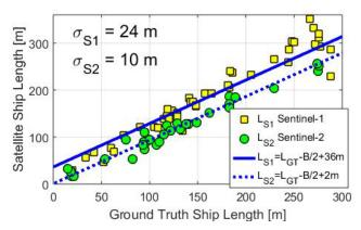
Figure 6. Ship lengths. Squares and circles are from S1 and S2 data respectively vs ground truth lengths and breadths from AIS ship records. Blue lines indicate best off-set fit to S1 data and dashed blue line to S2 data, see text.
