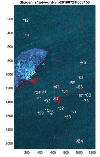
Figure 2. Copernicus Sentinel-1A image [August 21<sup>st</sup>, 2018 at 05:32 a.m. UTC] covering Skagen, the northern tip of Denmark. The added numbers refer to the list of objects found by the classification algorithm, where white numbers are ships and red numbers are mostly wakes, sidelobes, and harbor piers.
