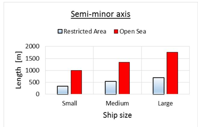
Figure 9. Length of semi-minor axis in restricted and open sea area for selected ships
