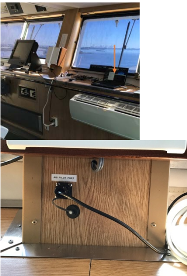
Figure 6. Left: Laptop (orange arrow) on ledge to the right of the pilot port (green arrow). Right: close-up of pilot port.
