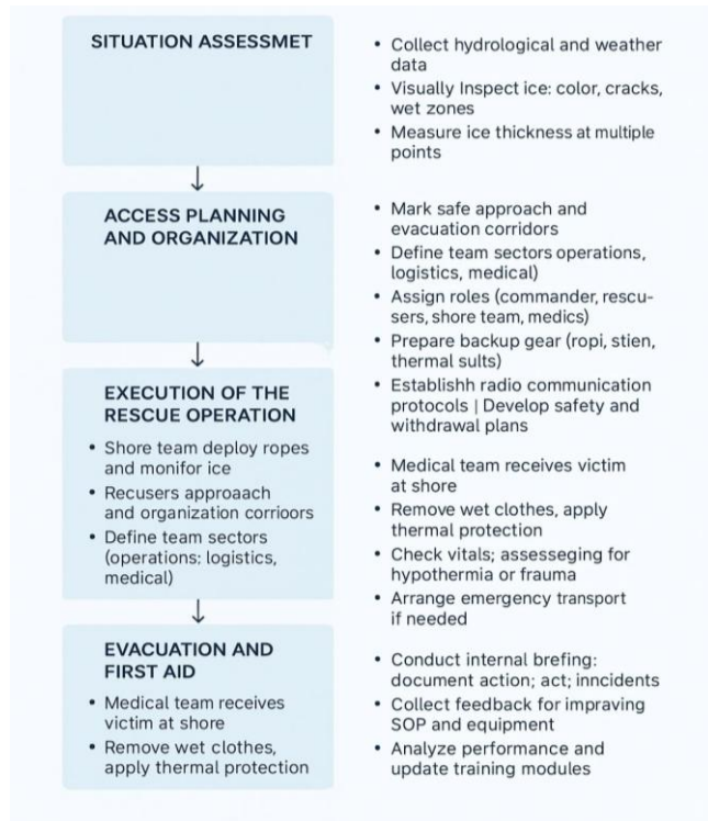
Figure 4. Algorithm: Standard operating procedures for ice river rescue operations
