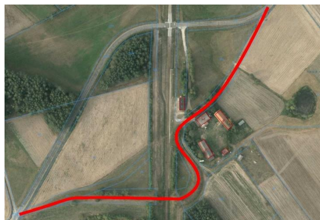
Figure 8. Proposal to replace the decommissioned 201 074 756 rail-road crossing with a rebuilt road viaduct at the Zielonka Pomorska passenger stop and to restore the historical alignment of the 1028C county road
