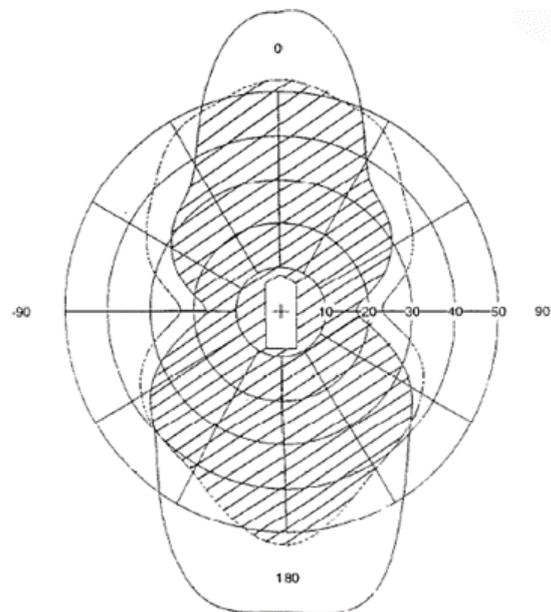
Figure 2. Typical DP capability plot diagram shape.
