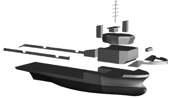
Figure 7. MWTO elements exposed to wind influence.
