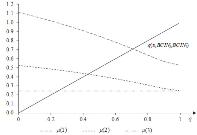
Figure 8. Mean values of the GBNCIN lifetimes in safety states subsets  $\{1, 2, 3\}$ ,  $\{2, 3\}$ , and  $\{3\}$ , given in years for coefficients  $q(v, BCIN_i, BCIN_i) = q$ ,  $i, j \in \{1, 2, \dots, 8\}$ ,  $v = 1, 2$ , ranging from zero to 0.99.
