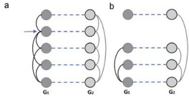
Figure 3. Mutual interactions of interdependent networks in case of nodes failures (Rueda and Calle 2017).
