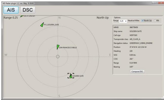
Figure 5. Screen shot of the AIS/DSC GUI window in AIS mode. M/v Golden Gate is the vessel to be called
