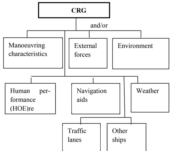
Figure 2. First level fault tree for CRG casualties
