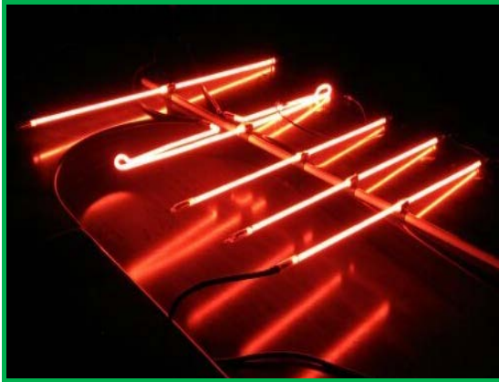
Figure 3/ Plasma Yagi antenna principle prototype
