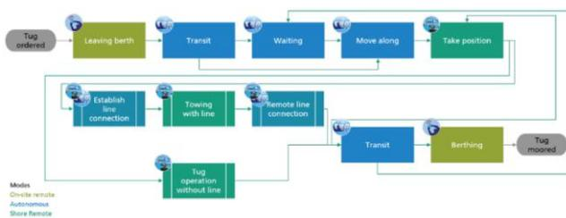
Figure 1. Flow chart for tug operation with remote FernSAMS assistance system [15]
