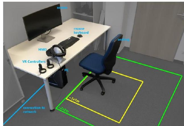
Figure 2. Shore Control Station Set Up
