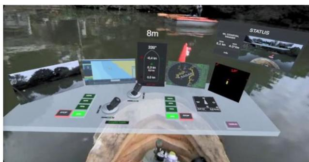
Figure 9. Virtual bridge with 360 degree-camera streaming
