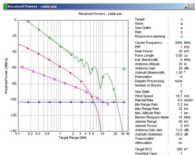
Figure 1. The course of object signal and noise for S band
