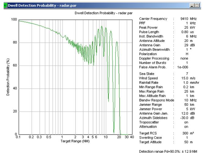
Figure 4. The probability of detecting X band radar
