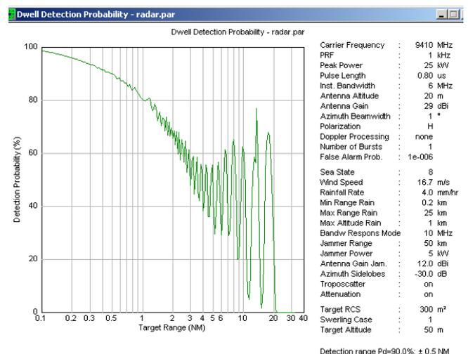
Figure 5. The probability of detecting band X radar
