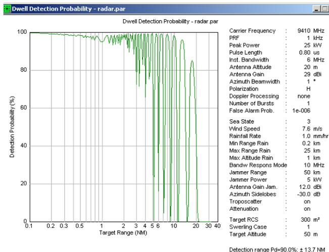
Figure 3. The distribution of probability of detecting a band X radar
