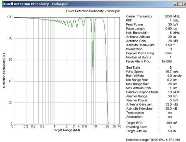
Figure 2. The distribution of probability of detecting a band S radar
