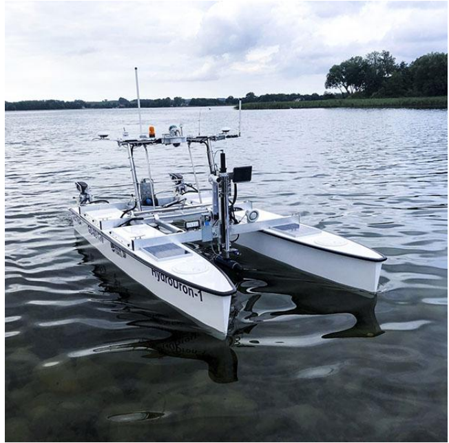
Figure 1. ASV HYDRODRON-1 by Marine Technology Ltd. used for the data acquisition
