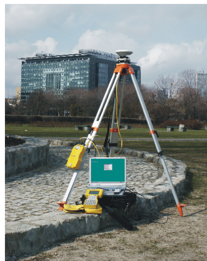
Fig. 1. Field set for RTK and DGPS measurements
