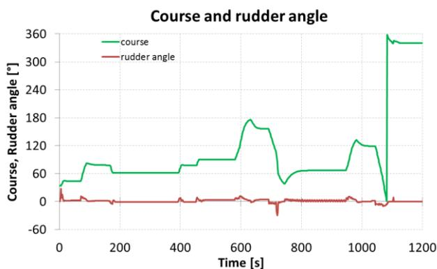
Figure 14. Plot of the course and the angle of the rudder of tug 1 - the leader of the formation.
