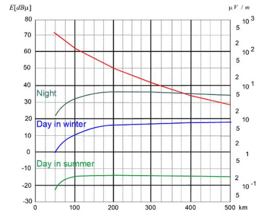
Figure 2. The signal strength for the surface wave and skywave as a function of the time of day and time of year, distance from the reference station for the frequency of 300 kHz and EPR of 1 kW. The red line denotes the signal strength for the surface wave [IALA, 1996].
