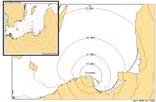
Figure 7. Signal strength level in  $\text{dB}\mu\text{V/m}$  for the Rozewie DGPS reference station [Specht, C., 2011].
