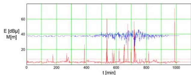
Figure 1. The signal strength - E [dBμ] (blue) of a Hoburg DGPS reference station and the mean positioning error - M ( $p = 0.95$ ) (red) as a function of time. Recording: 24-05-1995 11:50 UTC – 25-05-1995 04:50 UTC, Gdynia, measurement frequency: 1 minute [Specht, C., 1997].
