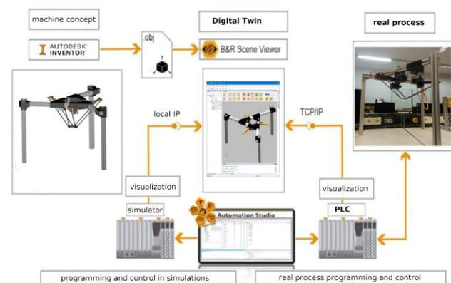
Figure 2. The principle of our solution using a digital twin
