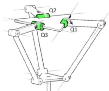
Figure 1. Three-axis parallel delta-type robot [2]
