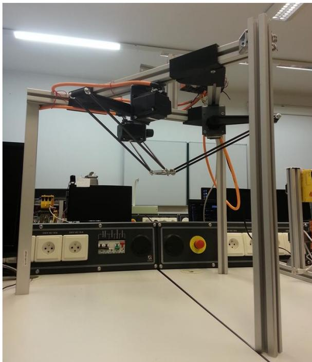
Figure 5. Our constructed delta robot
