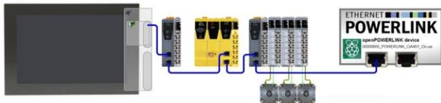
Figure 3. Hardware configuration in the Automation Studio
