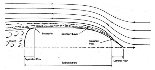
Figure 2. Flow pattern around a vessel in motion. [8, ch 7, p. 11]
