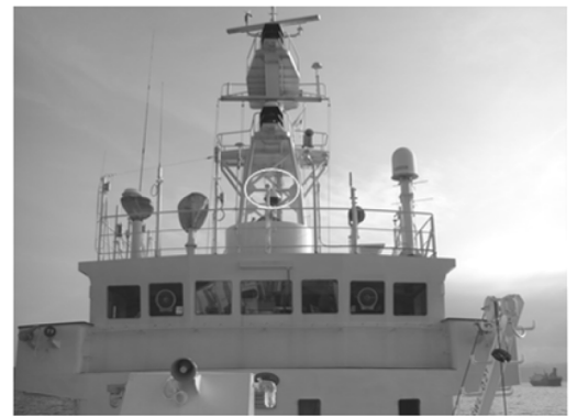
Figure 6. Arrangement on the Flying Bridge of T/S Shioji-maru. (VI-GPS ANT is shown in the white circle)
