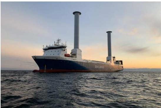
Figure 2. SC Connector – tilted rotors (Courtesy: SeaTrans Group)
