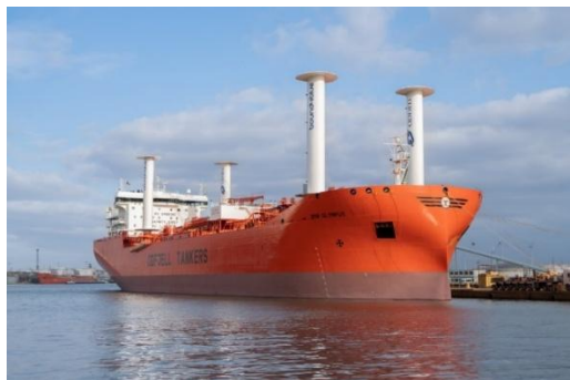
Figure 3. Bow Olympus – suction sails from Bound4blue installed (Courtesy Odfjell)
