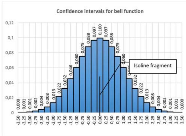
Figure 3. Histogram showing probabilities of the true isoline being located in the vicinity of the measured one
