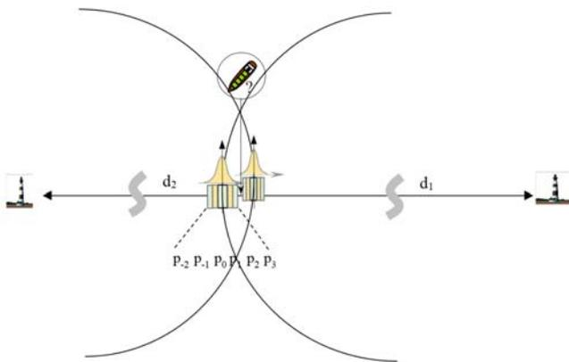
Figure 2. Graphical interpretation of two imprecise measurements, distorted with random and systematic errors, taken to objects at opposite directions
