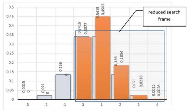
Figure 4. Histogram showing probabilities of the true isoline being located in the vicinity of the measured one and its modified version.
