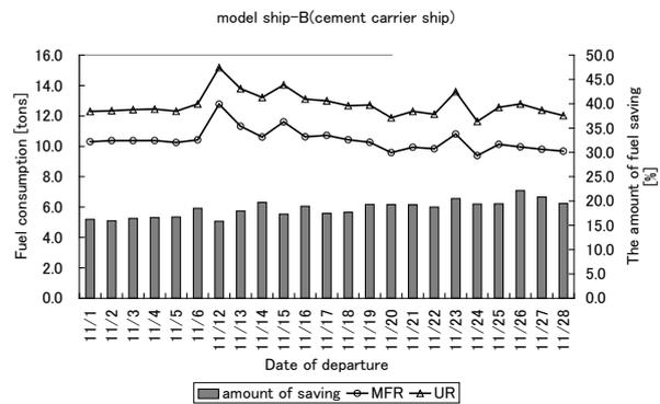
Figure 5. Fuel consumption and fuel saving amount for model ship-B.
