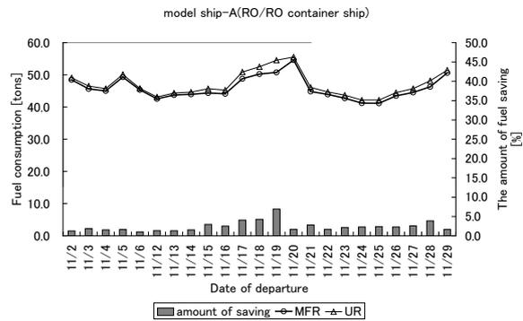
Figure 4. Fuel consumption and fuel saving amount for model ship-A.
