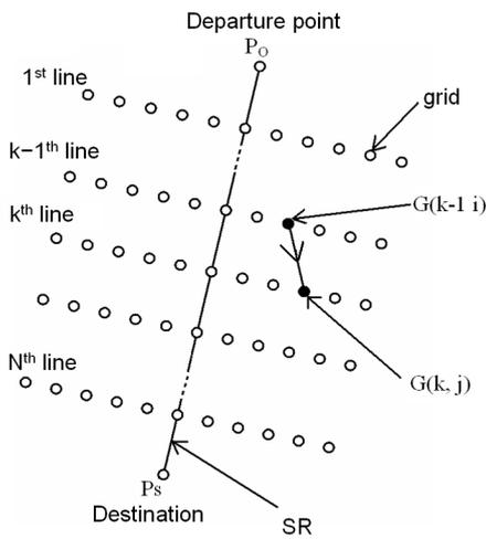
Figure 1. Grid points of DP to calculate minimum fuel route.
