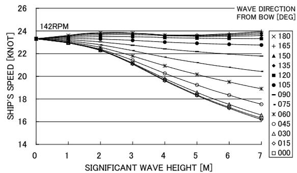
Figure 2. Speed performance curve of model ship-A at 142 RPM.
