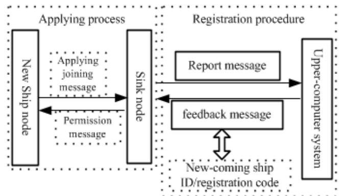
Figure 3. Schematic of new node joining into native sub-wsn
